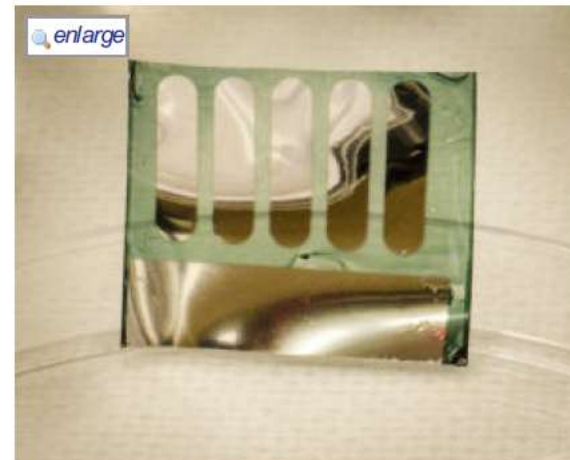
Photograph of a solar cell fabricated at Georgia Tech on nanocellulose substrates derived from trees. (Credit: Canek Fuentes-Hernandez, Georgia Tech)
